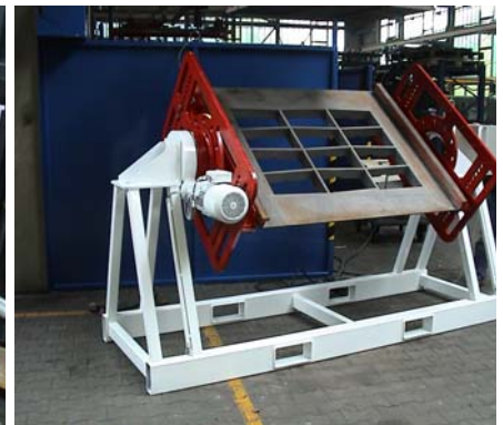
Positioning of the mould box in best position for maintenance work.
