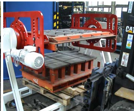
Stamp in upside down position taken away on a pallet by the forklift, mould box stays in mould turning device
