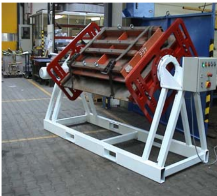
Mould box and stamp, strapped together with two security straps, fixed onto the mould turning device FW 1, turning has started.
