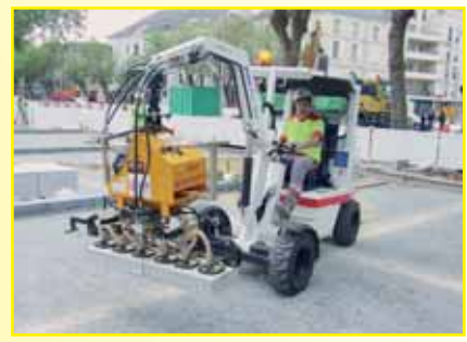
SH 1000 mini h, b or e , load classification up to 1,000 kg; powered either via hydraulic, petrol engine or electric power supply for slightly porous materials
