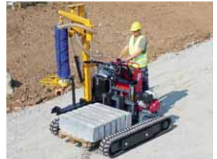
... laying of kerb stones: The smart choice with numerous advantages: With a standard trailer anywhere at any time - TRANS MOBIL TM.
